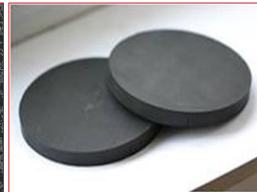
press and sintered metallurgical grade tantalum compacts
